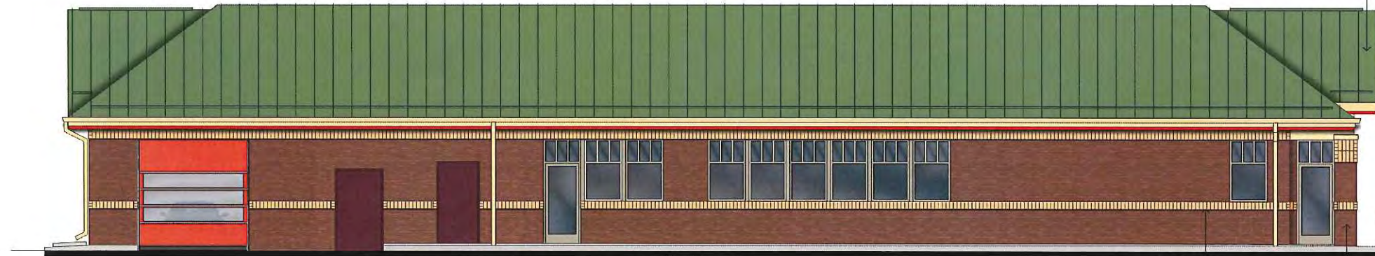
RED BRICK | TAN SOLDIER COURSE | TAN STUCCO | STANDING SEAM METAL ROOFING | FRONT ELEVATION 1/8" = 1'-0"
